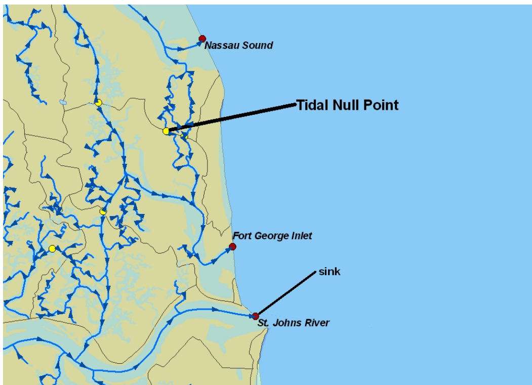
Figure 5. TidalNullPoints created for 3 of the 9 outlets along the Atlantic coast of the SJRWMD. The sinks used to determine flow direction during Arc Hydro network generation are also displayed.
